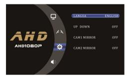
System setting: Language (English default), UP DOWN for display picture up and down change, CAM1 MIRROR and CAM2 MIRROR for Video1 and Video2 image mirrored and non-mirror display
